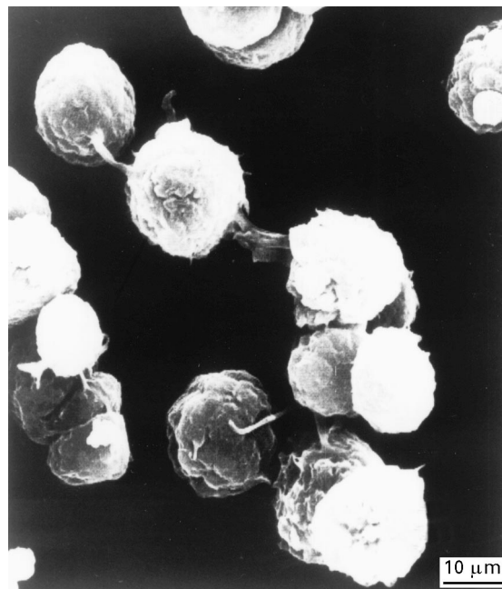
Figure 2 Scanning electron micrograph of pre-made PBT–PTMG copolymer powder.
